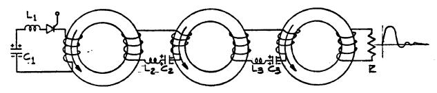
Discharge of C1 Drives First Out of Hegative Saturation, Transfers Energy To C2 CHARGING OF
