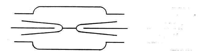
The idea is to use either this or a transformer pulse forming network. Simultaneity is important because without it you get reflections which bounce around and hurt you later (see sketch below using  $50 \Omega$ ):
