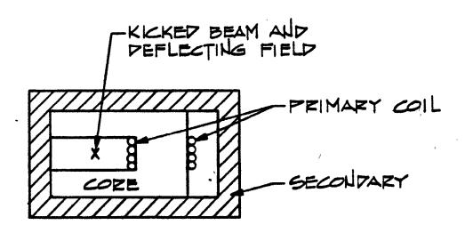
If this structure were surrounded by a superconducting box then the desired deflecting field would be produced in the gap when the primary is pulsed. This suggests that a grounded conducting box will contain the stray field for a limited time. This box is the secondary. Electrical considerations are
