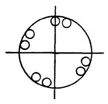
The separation shown in the above sketch is related to  $\delta$  in the tune, and as the filling of the outer part of the acceptance is done, then the injection angle and the parameter  $\delta$  are further adjusted to fill the inner part of the phase space as shown below.
