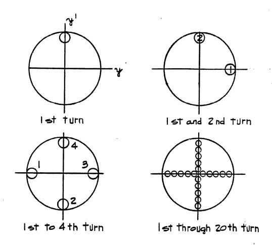
In the above sketch we assumed for simplicity that the space charge effect is turned off, and can conclude that the charge distribution in real space is lumpy.
