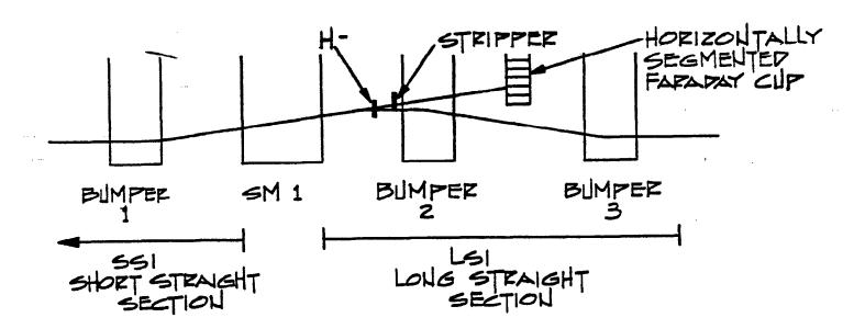
There are two 50% transparent Faraday cups situated in the L3 and L4 straight sections. The injection angle is adjusted by looking at first, second, and third turns.
