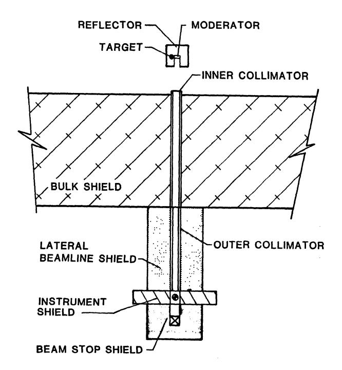
Fig. 1. Illustration of a typical beamline shield.
