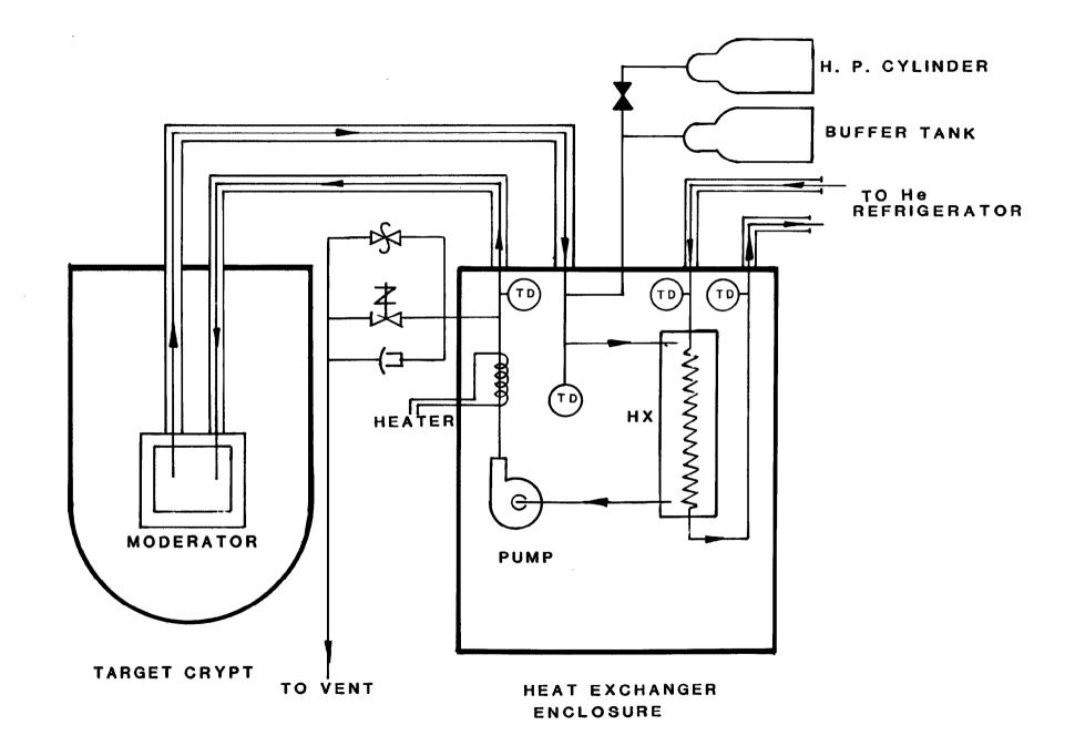
Figure 3. He/H<sub>2</sub> Heat Exchanger Schematic
