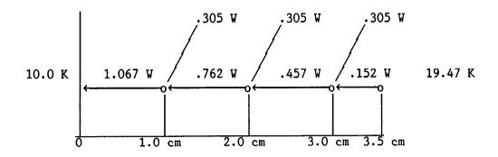
The calculation indicates that with a 6 % density, 10 PPI, 6101-T6 Duocel foam metal a maximum temperature of 19.47 K can be expected at the hottest point in the moderator. The moderator actually operates with the full heat load and with helium gas at 7 K, at a temperature of 12 K at the location of the thermocouple.
