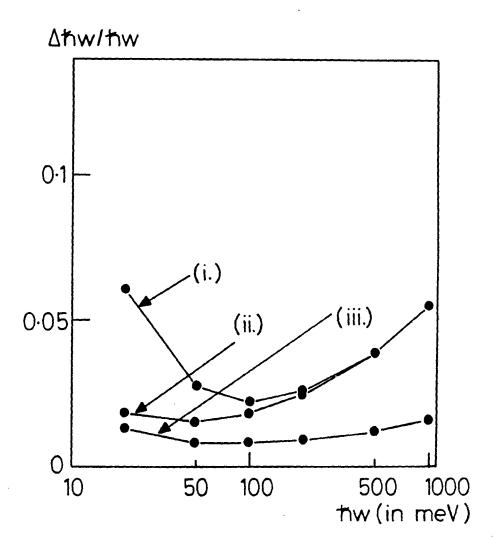
(2) Time focussed crystal analyser spectrometer energy transfer resolution  $\Delta h \omega / h \omega$  for (i) l" BF3 detectors, (ii) as (i) but with energy focussing and (iii) as (ii) but with an improved detector system.
