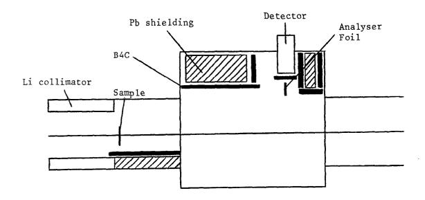
Figure 1b Internal shielding for scattering at 15°
