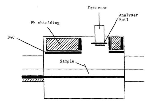
Figure 1a Internal shielding for scattering at 60°
