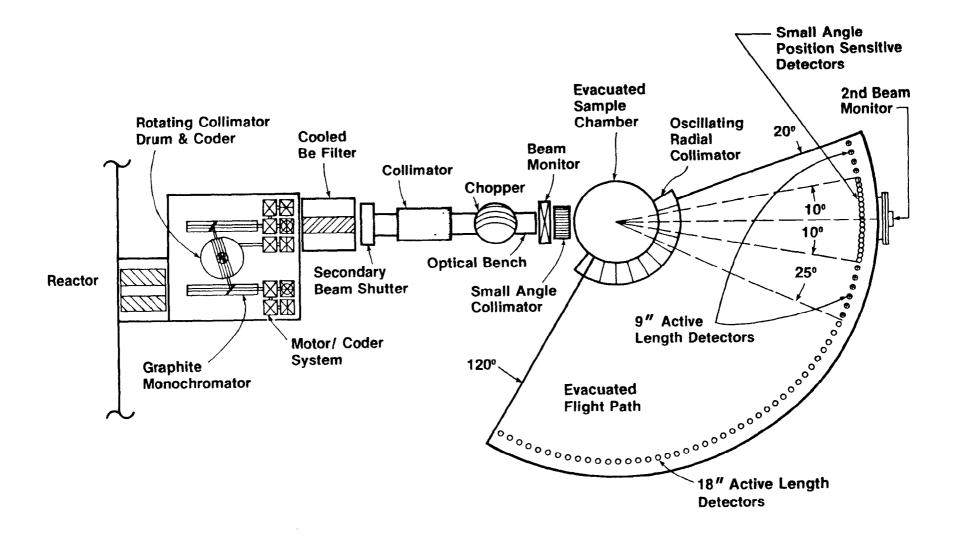
The NBS Neutron Time of Flight Spectrometer
