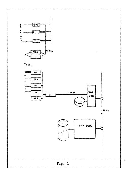
The shaded components indicate the points at which data is stored. In the DATA INPUT MODULES (DIM) the neutron event is time stamped and the time descriptor stored for up to  $5\mu s$  before being read out on the 10 MHz
