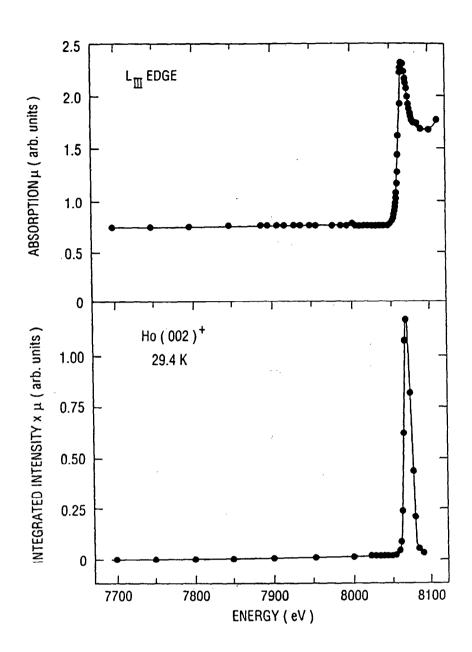
Fig. 2 Top: The absorption measured from a thin film. Bottom: The integrated magnetic intensity of the (002)+ reflection of Ho near the L<sub>III</sub> edge. After Gibbs et al. Ref. (4).
