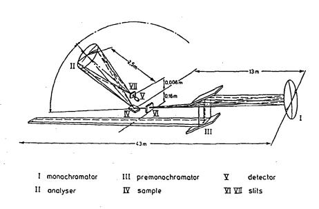
Fig. 3 Schematic setup of the instrument "INELAX" by Burkel et al (Ref 7).
