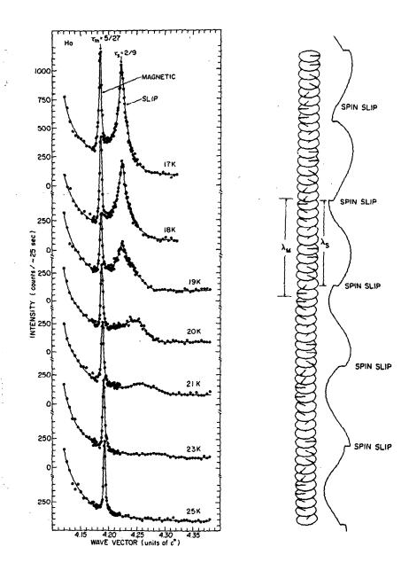
Fig. 1 Synchrotron x-ray diffraction pattern of the satellite above the (004) Bragg peak. The scattering pattern reflects both magnetic (5/27) and charge (2/9) modulations depicted on the spin slip model. After Gibbs et al. (Ref. 1)
