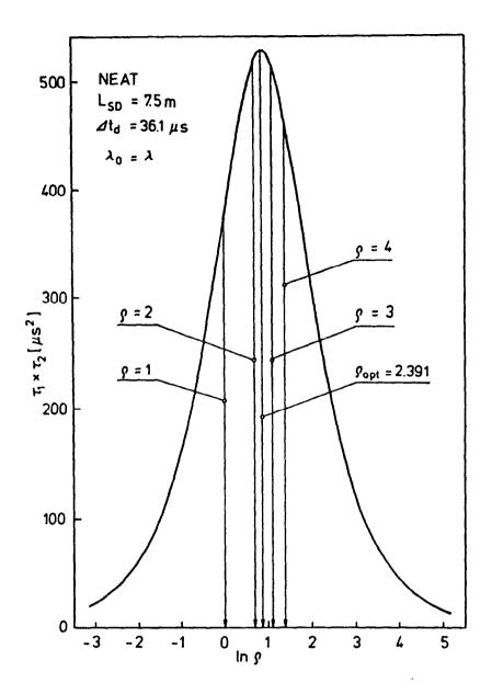
Fig. 3 Product of the chopper burst times  $\mathcal{T}_1 \cdot \mathcal{T}_2$  as a function of lno for the spectrometer NEAT with  $\lambda_0 = \lambda$ , sample-detector distance  $L_{SD}^{=}$  7.5m and time resolution  $\Delta t_d = 36.1 \ \mu s$ .
