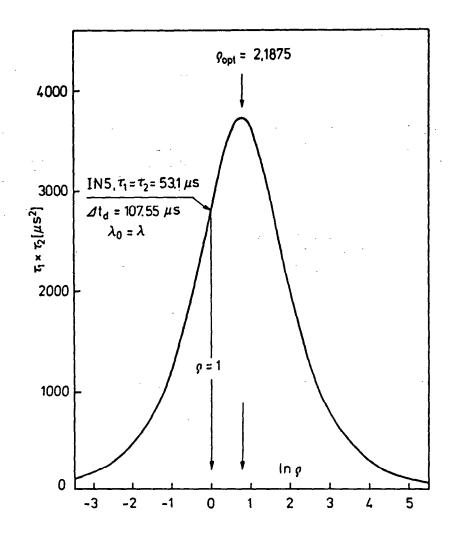
Fig. 2 The product of the chopper burst times  $\mathcal{T}_1 \cdot \mathcal{T}_2$  as a function of lno, where  $\mathcal{P} = \mathcal{T}_1/\mathcal{T}_2$ , is peaked at lno  $\mathcal{T}_1 \cdot \mathcal{T}_2$  is proportional to the intensity at the sample. Example: spectrometer IN5 for elastic scattering ( $\lambda_0 = \lambda$ ), for fixed time resolution at the detectors,  $\Delta t_d = 107.55 \,\mu s$ .
