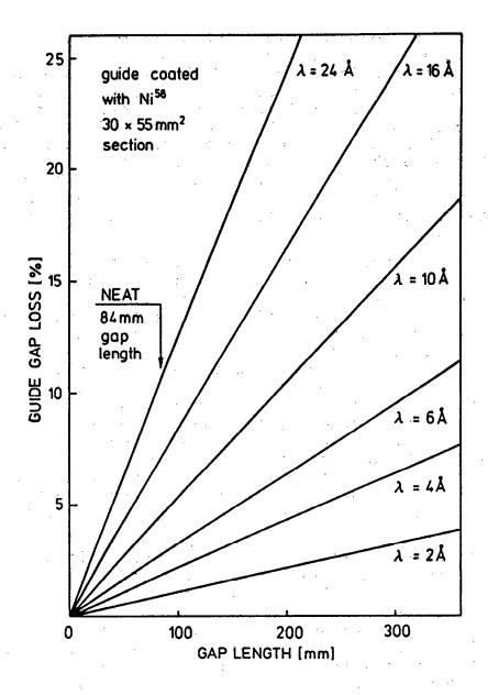
Fig. 7 Percentage of intensity loss due to interruptions in the neutron guide (guide gaps) as a function of the gap length, with the neutron wavelength  $\lambda$  as a parameter. The curves apply to the Ni-58 coated neutron guide section (with parallel, walls) of the spectrometer NEAT (beam cross-section: 30 X 55 mm<sup>2</sup>).
