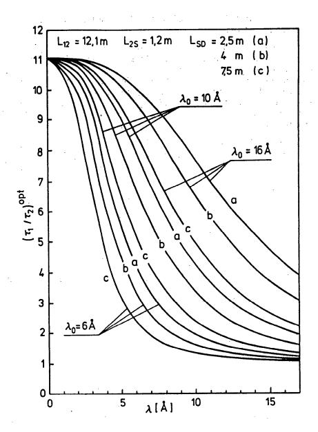
Fig. 4 Optimum burst-time ratio  $\rho_{\mathrm{Opt}} = (\mathcal{T}_1/\mathcal{T}_2)^{\mathrm{opt}}$  of the spectrometer NEAT as a function of scattered neutron wavelength  $\lambda$ , with incident neutron wavelength  $\lambda_0$  and sample-detector distance  $L_{\mathrm{SD}}$  as parameters.  $L_{\mathrm{12}} = \mathrm{distance}$  between the two principal choppers,  $L_{\mathrm{2S}} = \mathrm{distance}$  from the last chopper to the sample.
