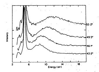
Figure 2. Recoil scattering from KHCO<sub>3</sub> with momentum transfer along the hydrogen bond. Scattering from hydrogen occurs at high energies/short times and is well separated from that due to heavier atoms.
