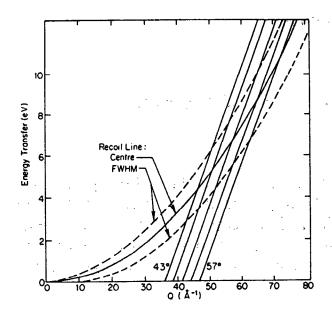
Figure 1. Time-of-flight loci from the 4.906 eV Au resonance analyser used in the momentum distribution measurements on a single crystal of KHCO<sub>3</sub>.
