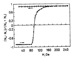
Fig.2. The experimental dependence of  $P_o \cdot P_m(H) = \frac{N_+ - N_-}{N_+ + N_-}$  on the external magnetic field parallel to the "easy axis" of the anisotropic FeCo film. At first the film was magnetized in the opposite direction to the external magnetic field. The reversal of magnetization of the film leads to the changing of sign of film polarizability.
