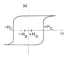
Fig.1. The typical magnetization reversal curve of a single-axis anisotropic film, when the magnetic field is directed to the "easy axis" of anisotropy of a film. In the region  $-H_o < H < H_o$  the dependence of the magnetic moment  $\vec{M}_p$  of a film on the volume and direction of an external magnetic field H is absent.
