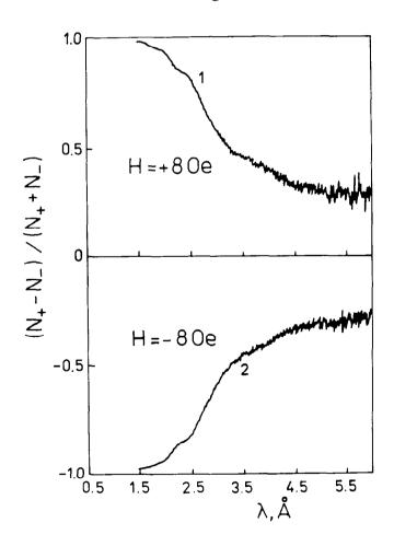
Fig.3. The experimental wavelength dependence of  $P_o \cdot P_m(H) = \frac{N_+ - N_-}{N_+ + N_-}$  for the FeCo single-axis anisotropic film: curves 1,2 correspond to the magnetic field equal to +8 Oe and -8 Oe, respectively. The changing of sign of the external magnetic field leads to the changing of sign polarizability of the film in a wide range of the wavelengths.
