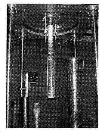
thermocouple located inside the sample volume and typically in contact with the sample. Due to the scattering geometry, only 90° scattering angles are available with the Miller furnaces; therefore, the only compatible instruments are the GPPD and SEPD.
