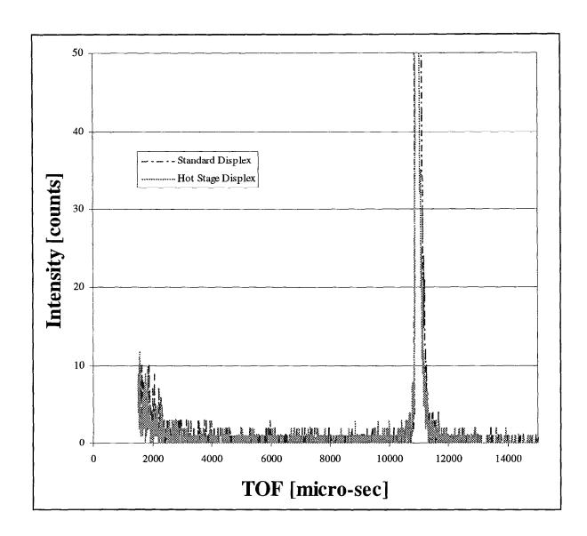
Figure 4. Comparison of raw TOF data taken on QENS with the Hot Stage Displex® and with a standard Displex®. Though the two plots are of different samples, the backgrounds of the two plots in the 1500 - 15000 µsec range are comparable and quite good.
