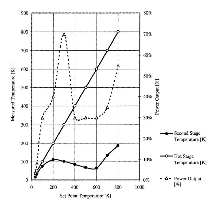
Figure 3. Heating plot of second stage temperature, Hot Stage temperature, and percent power output to heater as a function of Hot Stage set point.
