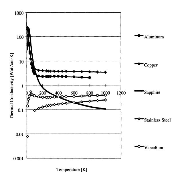
Figure 2. Thermal conductivity<sup>12</sup> of single crystal sapphire plotted along with that of aluminum, copper, 304 stainless steel, and vanadium.
