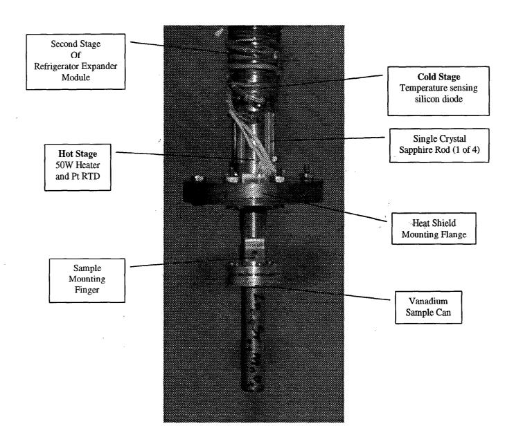
Figure 1. The Hot Stage Displex®. The sample can show is a low temperature indium o-ring sealed vanadium sample can of the type that is usually used in low temperature measurements on the powder diffractometers. A similar sample container with a flange capable retaining a helium leak tight seal throughout the temperature range of the Hot Stage is being developed.
