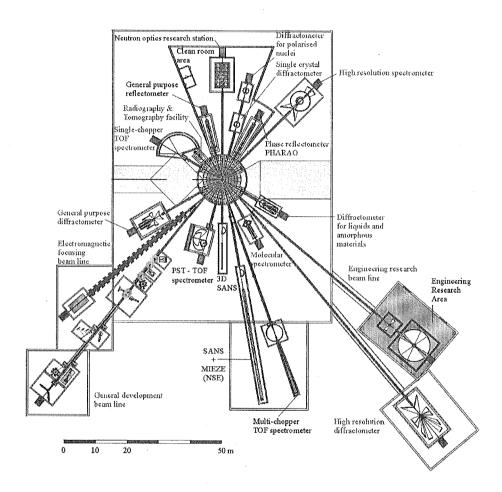
Figure: Proposed Layout of AUSTRON instruments; see Table for details
