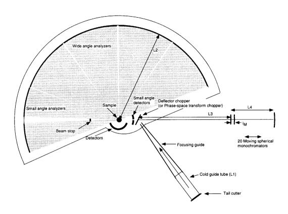
Figure 1: Schematic drawing of the Doppler-Musical spectrometer.
