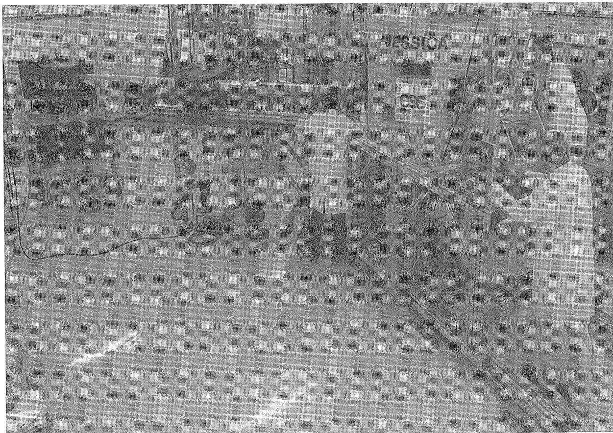
The JESSICA facility: proton beam line (from top centre), reflector vessel with target and moderator and primary neutron flight path (between reflector vessel and black detector box)
