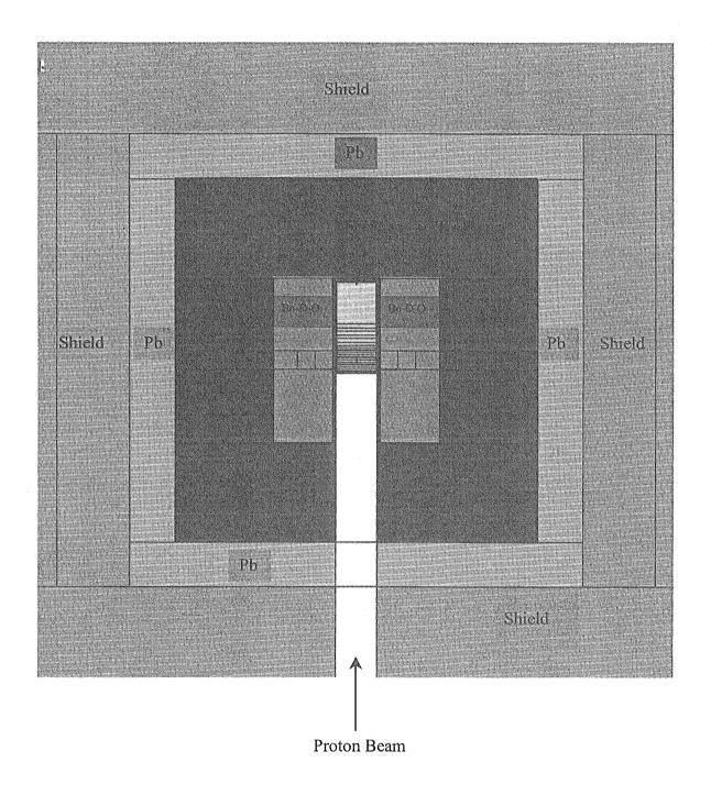
Figure 3: Spallation Only Neutron Source
