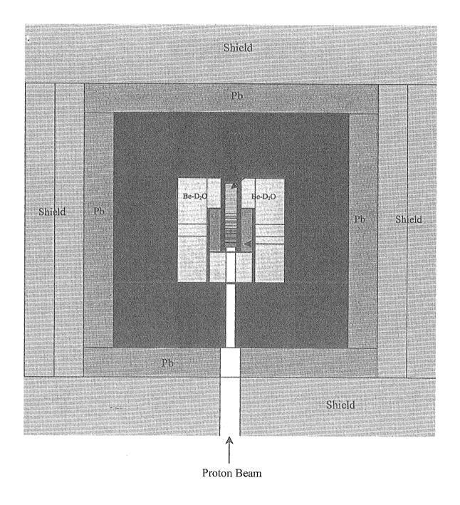
Figure 2: Spallation Neutron Source Surrounded by a Fissile Blanket
