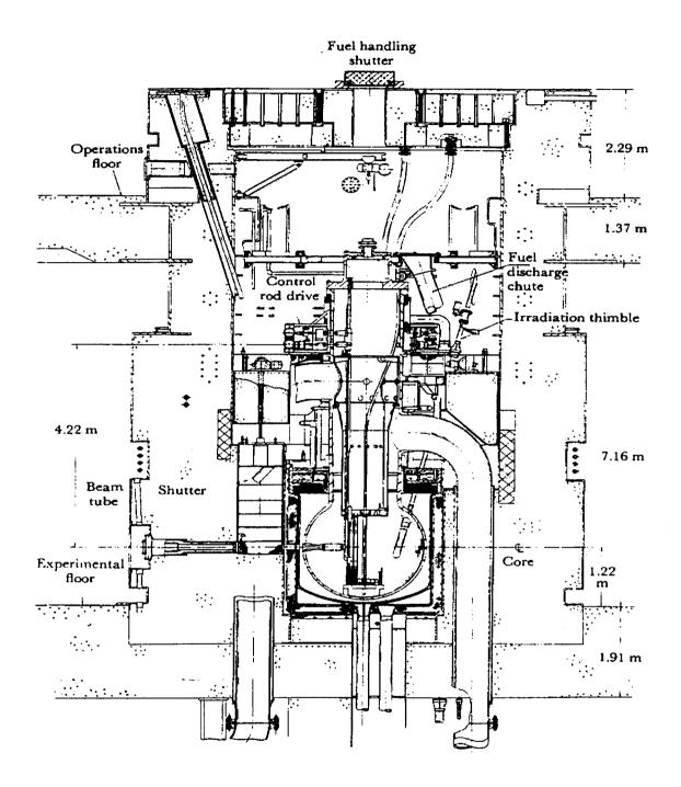
Figure 1: Elevation of the Reactor Vessel Shielding, Showing a Typical Beam Tube, Shutter, and Thimble
