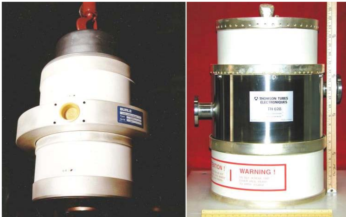
Fig. 2. The existing 201 MHz 7835 triode on the left and the proposed TH628 Diacrode® on the right.
