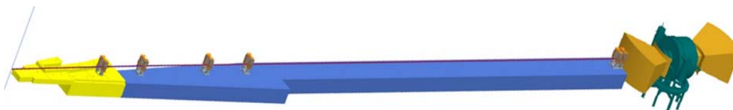
Figure 1. CAD model of the ZEEMANS instrument. Showing (From the left to the right), The neutron guide, the 4 bandwidth choppers, two high-speed choppers the backward scattering detector bank, the magnet on the rotation stage and the forward scattering detector bank.
