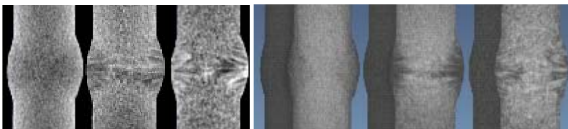
Fig. 8. Energy selective tomography of the welded stainless steel sample. Left: Reconstructed slices from the bulk of the sample in the polychromatic beam (left), at 4.1 Å (middle) and at 3.5 Å (right). Right: Reconstructed volumes in the polychromatic beam (left), at 4.1 Å (middle) and at 3.5 Å (right).
