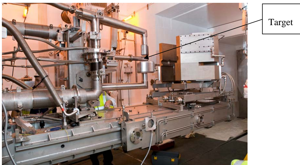
Fig 2. The Target, Reflector and Moderator Assembly in maintenance position
