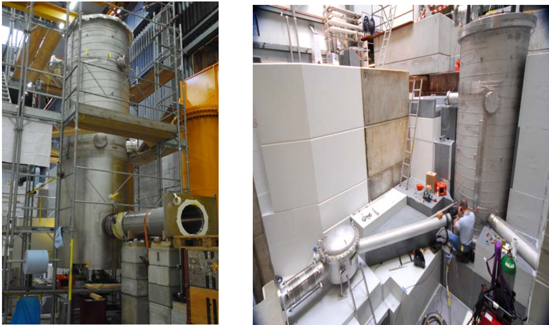
Figure 2: The UCN tank housing the D_2O moderator vessel and (later) the UCN storage volume. Left: shortly after delivery to PSI, with the target insertion tube still visible. Right: At its final position, partly surrounded by shielding, with the lower neutron guide channels mounted.
