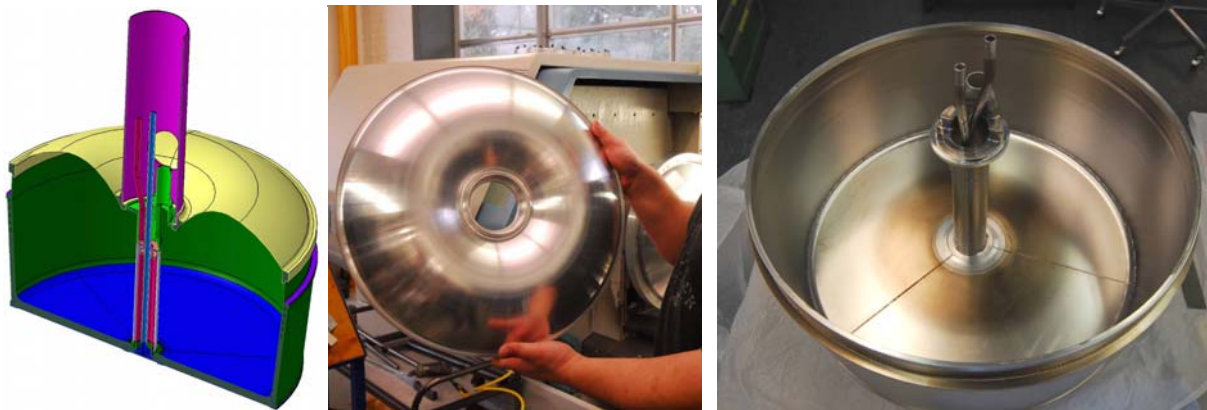
Figure 4: Design drawing (half-cut) of the sD 2 moderator vessel (left), the donat-shaped top lid (centre) and vessel body with the liquid D 2 and He feeding pipes in the centre (right).
