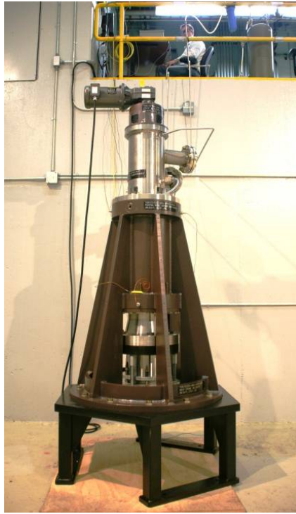
Figure 3. Full-scale rotating target drive module.
