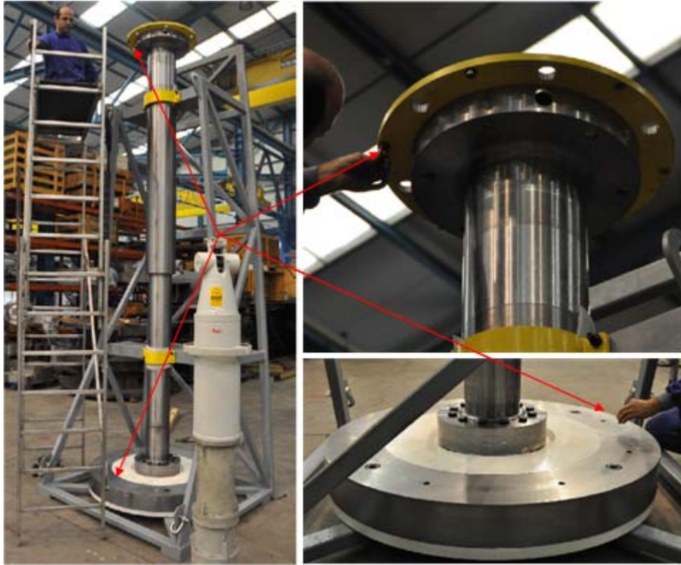
Figure 2. Laser tracker measurements on target module assembly performed to double check the validity of clock gauges measurements on horizontal setup.
