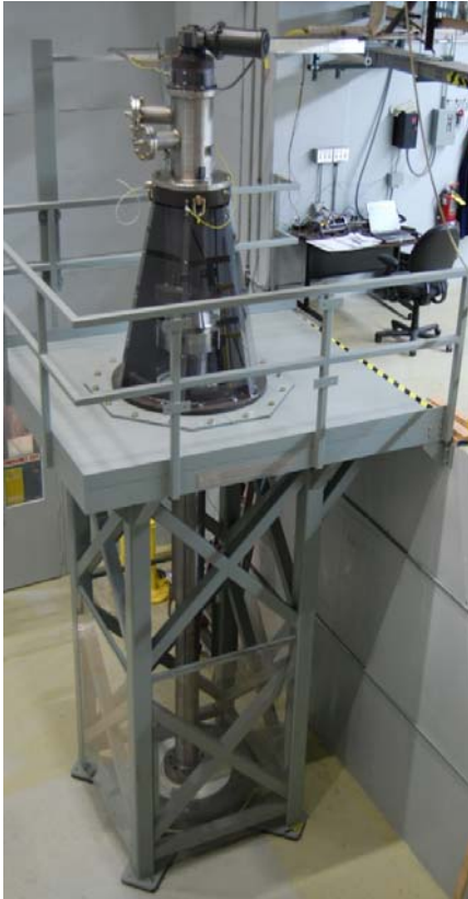
Figure 4. Full-scale, prototypical rotating target mockup assembly.
