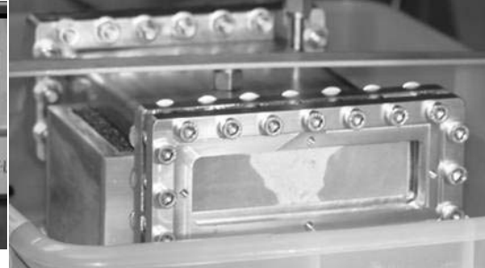
Fig. 3 Pre-irradiation testing of texture enhanced gas wall target with acrylic version of beam window.
