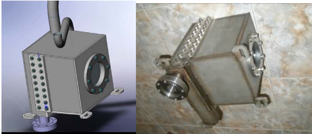
Fig. 6. Cold moderator chamber without vacuum jacket. a) Model, b) Manufactured
