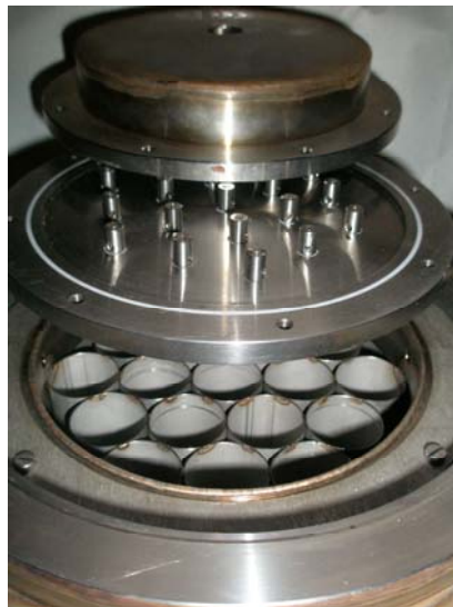
Fig. 7. The device for mesitylene balls preparation (a vacuum housing is removed).
