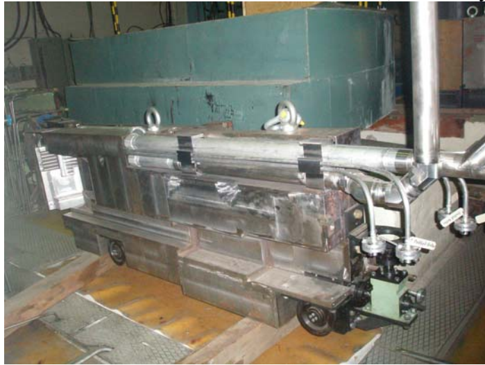
Fig.1. The chamber of cold moderator with a special trolley of biological shield of the IBR-2M reactor
