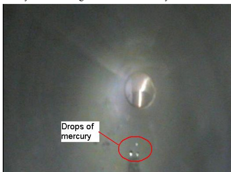
Fig. 2 Photograph of inner surface of the pipe in the mercury circulation system. Some drops of mercury are seen, but nothing special is found.
