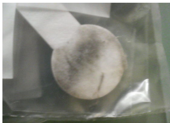
Fig. 3 Photograph of a piece of paper smeared inner surface of the pipe of mercury circulation system.
