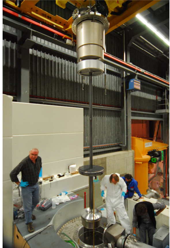
Figure 3. Insertion of the moderator unit into the UCN vacuum tank. The SD2 moderator vessel can be seen at the lower end.
