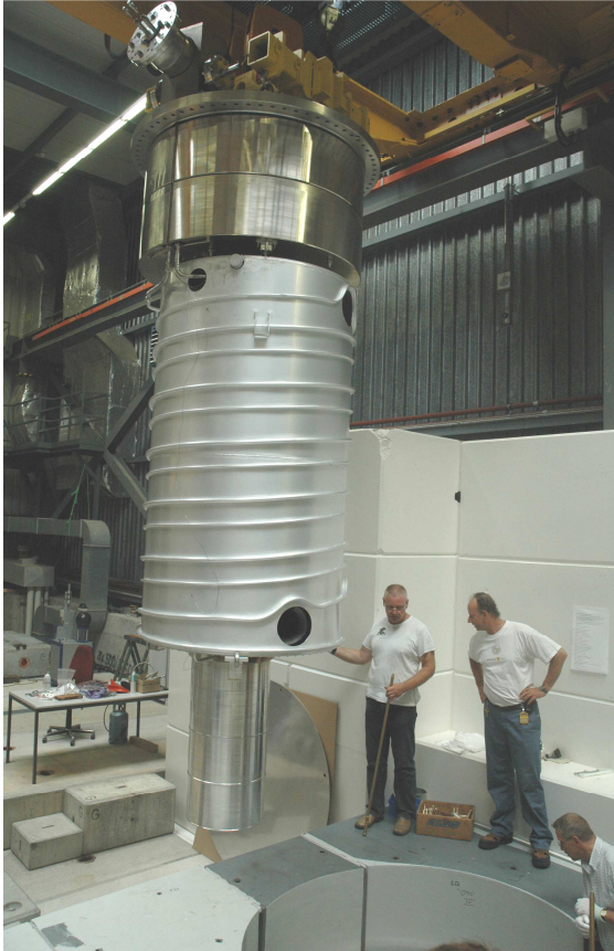
Figure 2: The storage volume inside the thermal shield before insertion into the vacuum tank.
