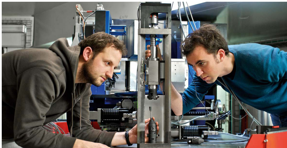
Figure 4: Two young scientists at PSI adjust a tensile sample inside a mechanical load frame installed at the POLDI instrument. These in-situ experiments provide an insight into the deformation behavior of metals and alloys by means of neutron diffraction.
