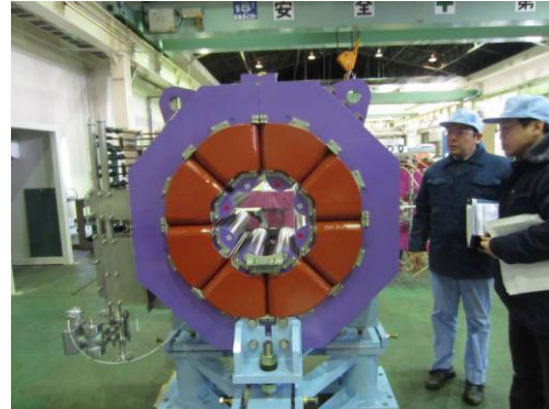
Figure 7 Octupole fabricated for the beam flattening system
