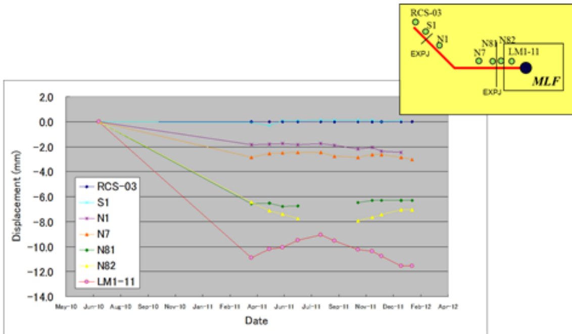
Figure 9 Trend of floor level after the earthquake on Mar 11th 2011 based on the result measured in Jun 2010. The observed position is shown in right upper side.
