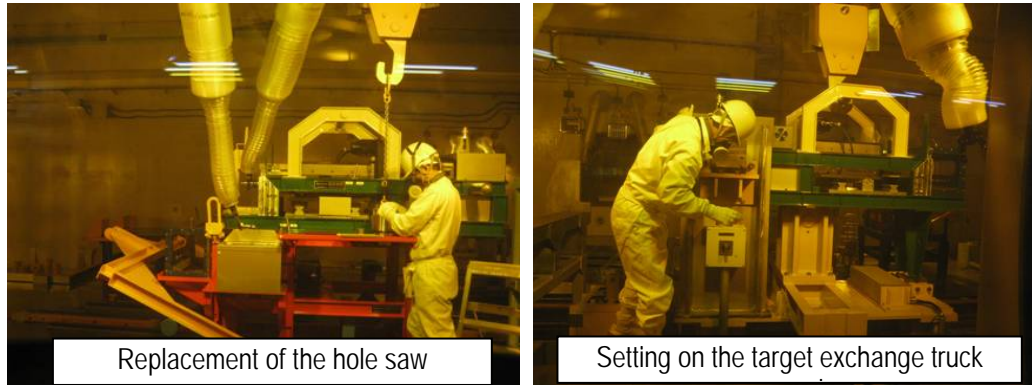
Figure 7. Photos of remote handling test in the hot cell
