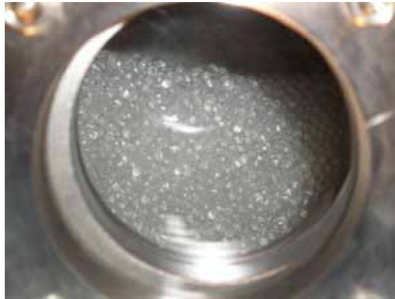
Figure 3. Photo of the cold solid beads of mesitylene at T \sim 40\text{K} inside the chamber-imitator of the moderator chamber.
