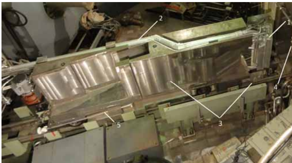
Figure 5. Moveable trolley with cold moderator and biological shielding installed in the rails in ready to move to active core position. (1- cold moderator with vacuum shielding and water pre-moderator, 2- cold helium and beads support pipelines, 3- trolley onto the rails, 4 - the entrance of passing through the stationary biological shielding of reactor to the active core, 5- drain pipeline of liquid mesitylene)
