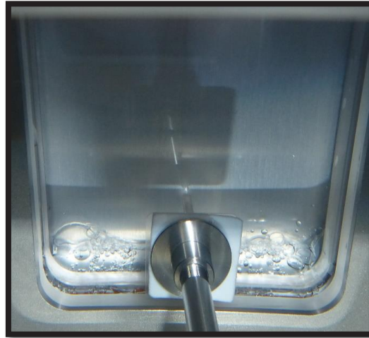
Figure 6. Incoming water helium solution evaporates due to the vacuum. Helium frees itself from the solution and can be measured
