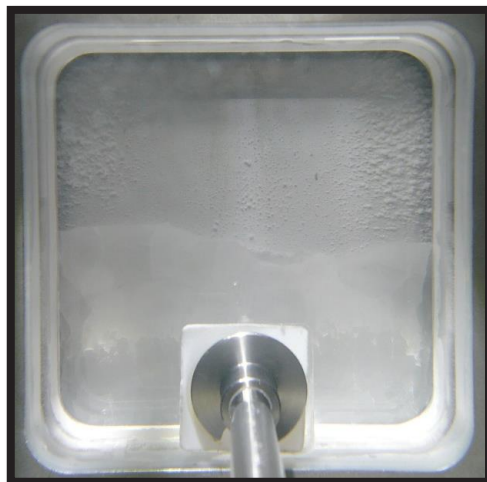
Figure 7. On the cold surface of the "moderator" frozen water. Helium diffuses through the ice and can be measured
