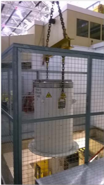
Figure 17(Left) – Loaded flask being lifted clear of services tunnel & Figure 18 (Right) – Flask being transported to R40 for short term storage
