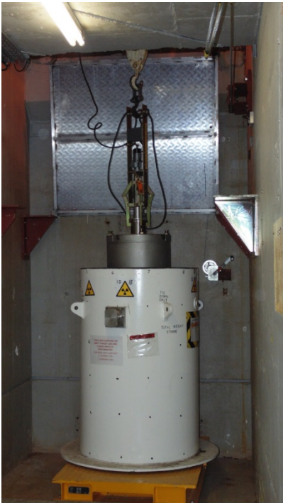
Figure 15 (left) shows target in Disposal Can being lowered into storage flask & Figure 16 (right) shows loaded flask being checked for external radiation dose
