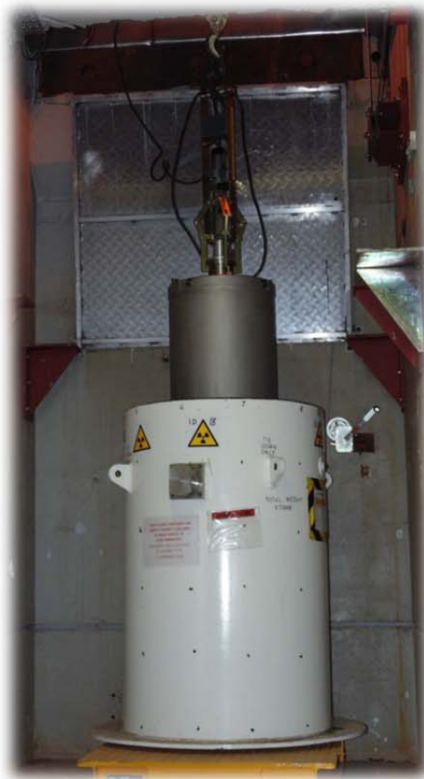
Figure 6 – Storage flask shield plug being lifted into RHC
