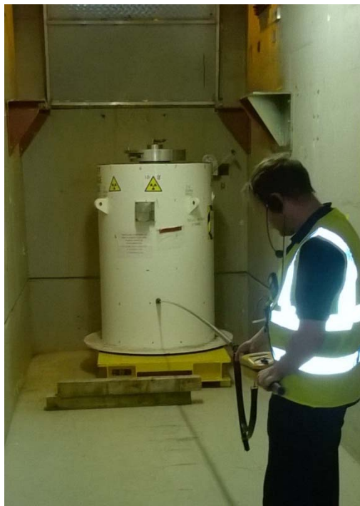
Figure 15 (left) shows target in Disposal Can being lowered into storage flask & Figure 16 (right) shows loaded flask being checked for external radiation dose
