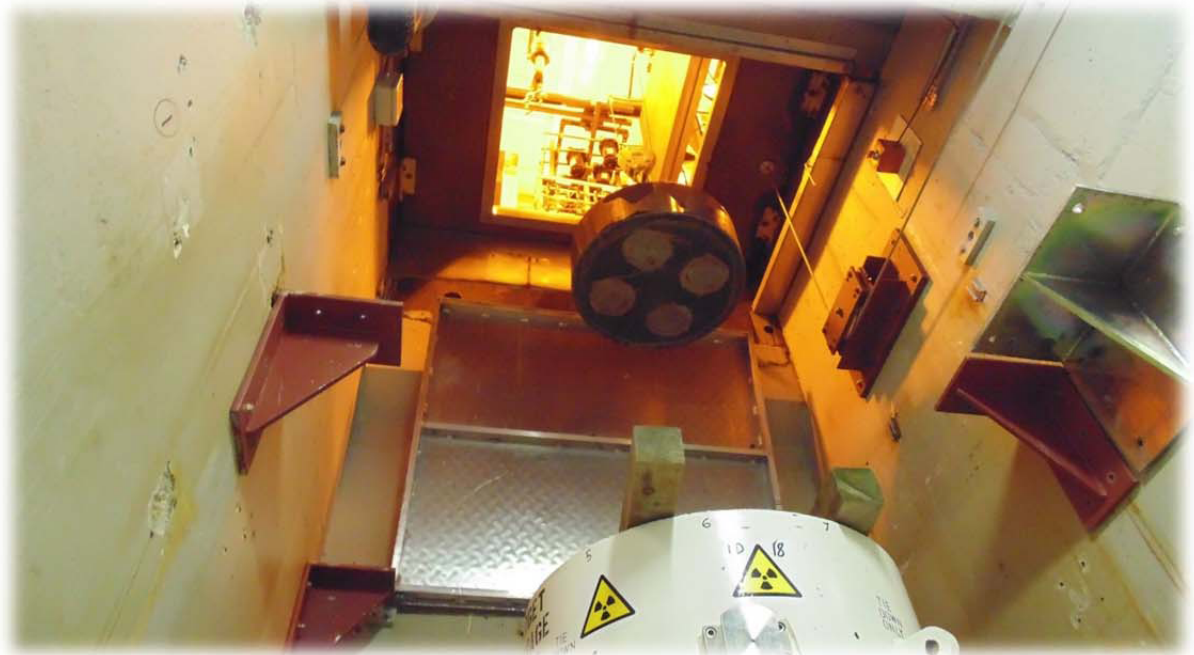
Figure 6 – Storage flask shield plug being lifted into RHC
