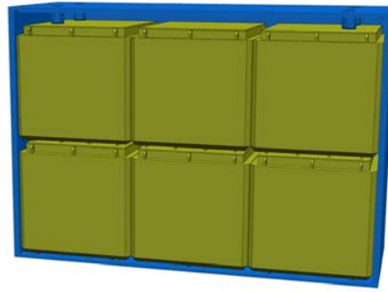
Figure 7. Detail of the waste shipment container (blue), one side omitted. The yellow wastebaskets are used as interim storage baskets that are eventually loaded inside the shipment container.
