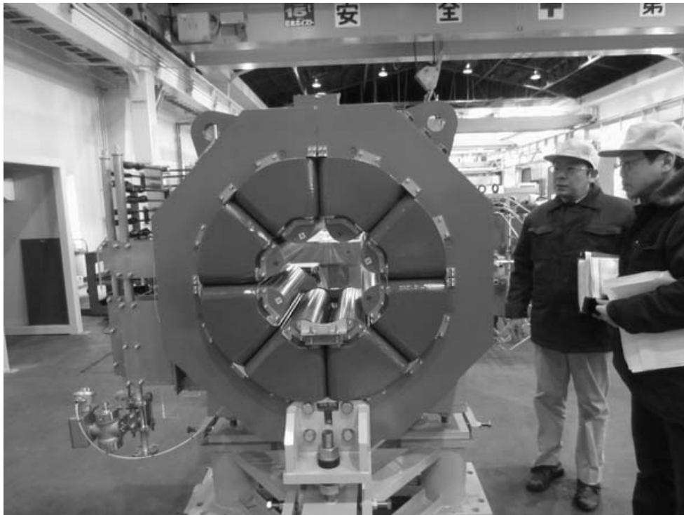
Figure 5: Fabricated octupole magnet with magnetic field gradient of 800 \text{ T/m}^3 .
