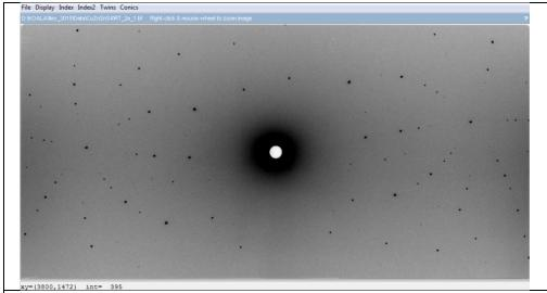
**Figure 2.** Example of Laue data obtained using KOALA (ANSTO) on a single-crystal sample of Cu<sub>2</sub>ZnSnS<sub>4</sub>.
