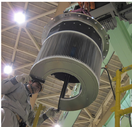
Figure 7. MLF technical staff installing the radial collimator on 4SEASONS.
