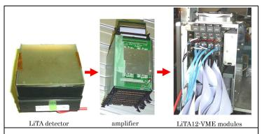
**Figure 1.** Block diagram of the LiTA12 system with a no-cut scintillator detector for the exclusive function.
