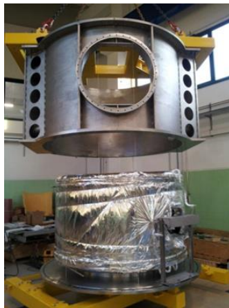
Figure 5. Assembly of vacuum container around cold mass
