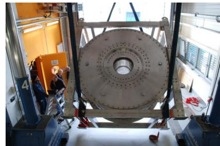
Figure 6. Rotation of magnet to orient magnet axis horizontal
