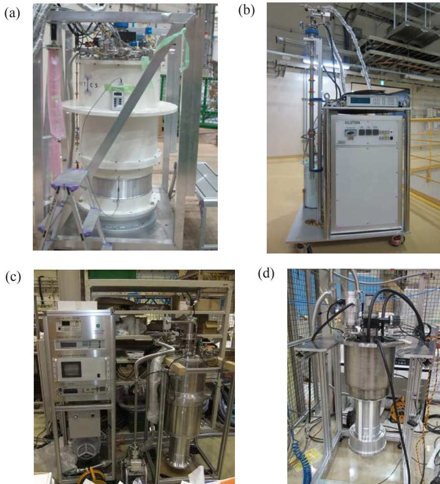
Figure 3. BL-common SE equipment managed by the SE team. (a) Vertical-field superconducting cryomagnet, (b) ^3\text{He} - ^4\text{He} dilution refrigerator insert, (c) top-loading-type ^4\text{He} cryostat and (d) High-temperature furnace with a Nb heater.
