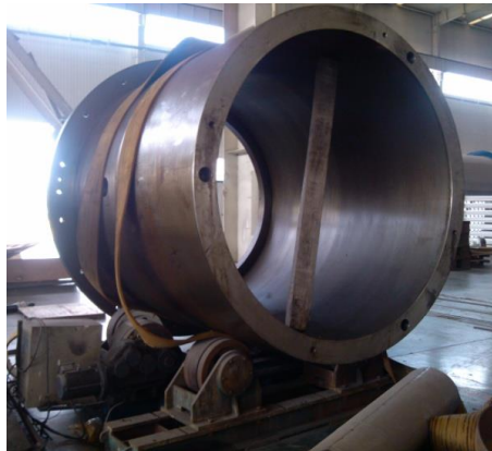
Figure 9. Support skirt roundness correction
