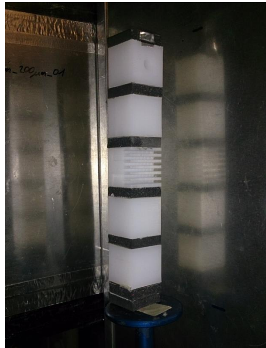
Figure 3. Examples for configurations with two (left) and one (right) specimen. In standard radiography set-ups (left) the detector (scintillator and CCD camera) is behind the samples and the neutrons illuminate the two columns simultaneously. With the detector sideways (right) only one column could be investigated at a time. Some of the measurements with one column included detectors both behind and on the side. The single column (right) is mirrored in the detector behind it and in an imaging plate at the side. From these optical reflections by plane surfaces an assessment concerning the alignment (e.g. tilt) of the columns can be drawn.
