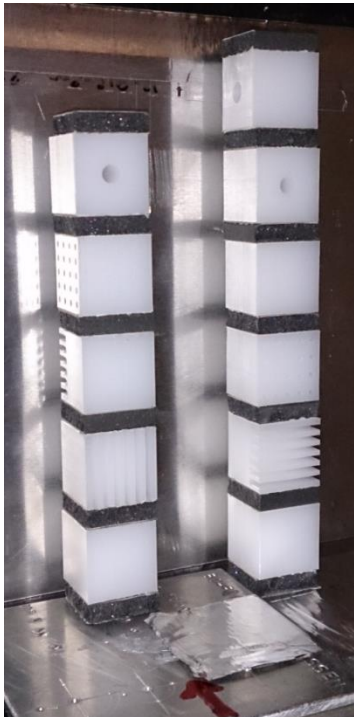
Figure 3. Examples for configurations with two (left) and one (right) specimen. In standard radiography set-ups (left) the detector (scintillator and CCD camera) is behind the samples and the neutrons illuminate the two columns simultaneously. With the detector sideways (right) only one column could be investigated at a time. Some of the measurements with one column included detectors both behind and on the side. The single column (right) is mirrored in the detector behind it and in an imaging plate at the side. From these optical reflections by plane surfaces an assessment concerning the alignment (e.g. tilt) of the columns can be drawn.
