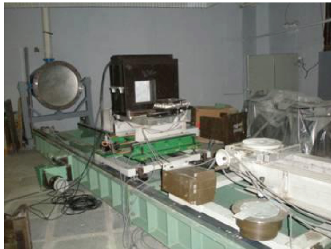
Figure 2. PSD in shield is installed on 8 th channel.
